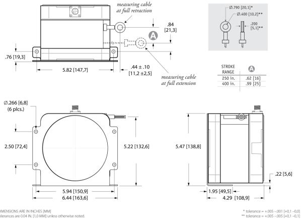
DIMENSIONS ARE IN INCHES [MM] tolerances are 0.04 IN. [1,0 MM] unless otherwise noted.
