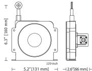
The economically priced SGJ provides linear position sensing over J1939 CANbus for OEM, mobile equipment and factory automation applications. Designed to withstand IP67 environments, the SGJ is constructed with a rugged polycarbonate body, an extremely durable spring-loaded stainless steel measuring cable and a stainless steel mounting bracket. For the OEM, customized options are available.
