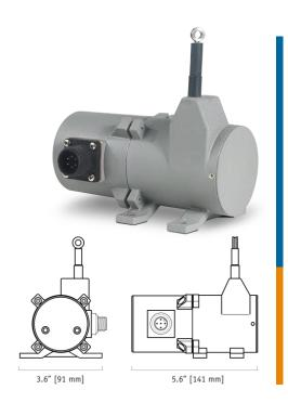
The PT8DN, using a high cycle plastic-hybrid potentiometer, communicates via DeviceNET protocol with programmable controllers in factories and harsh environments requiring linear position measurements in ranges up to 60".
