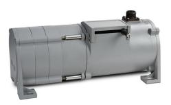
The PT9101 is a work-horse for demanding long-range applications requiring a linear position measurements in ranges up to 1700 inches. Available with either a 500, 1K, 5K, or 10K ohm potentiometer, the PT9101 operates with any basic panel meter or programmable controller.
