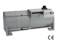
The PT9510 can operate from an unregulated 14.5 to 40 VDC power supply while providing a regulated output signal over its full extended range of up to 1700". It provides a 0 - 10 VDC position feedback signal proportional to the linear movement of its stainless steel measuring cable.
